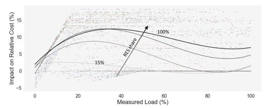
**Figure 12.** The impact of Dummy Charging on the total cost. It presents the simulations of numerous scenarios considering various environmental conditions and load profiles, for different level of load passing through control reference point (hybrid inverter) in case of dummy charging (represented by the points in the background), and the second-order interpolation of the obtained results in terms of relative cost versus no-battery case.
