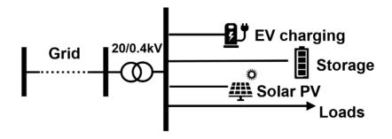
Figure 1. Component-wise view of use-case's local system.
