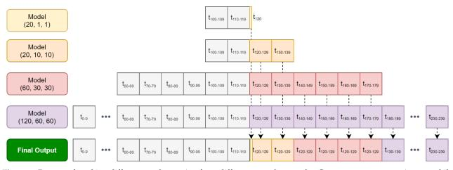
**Figure 7.** Process of stacking different results coming from different neural networks. Grey squares represent inputs, while yellow, orange, red, and purple squares denote outputs for each model denoted by corresponding triplet (I, O, F). Last line outlines final output, concatenation of all different contributes.
