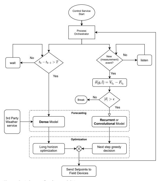
Figure 2. Logical process flow for control chain.
