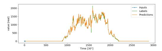
**Figure 8.** An example of performance of the WaveNet (20, 1, 1) architecture on a test data window. These data represent solar irradiance of a single day predicted by iteratively taking into consideration rolling input data and using output to predict a single future value.
