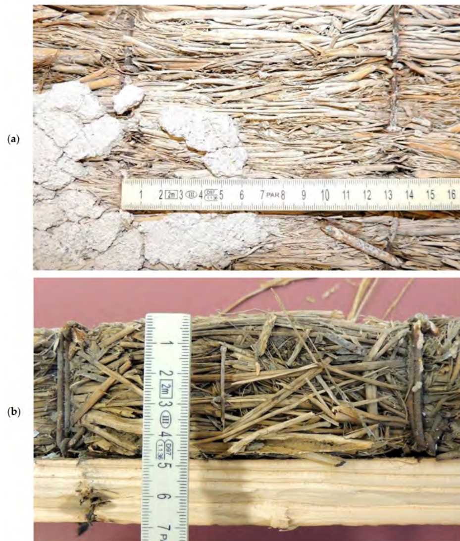
Figure 5. The tested SOLOMIT sample—cut rapeseed straw, binding with steel staples and the remains of the wooden structural frame and plaster: (a) surface of the panel, and (b) cross-section of the wall.
