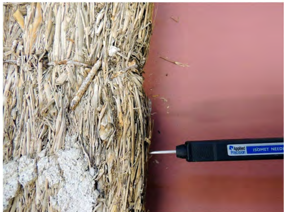
Figure 7. Needle sensor pressed into the material during the measurement.
