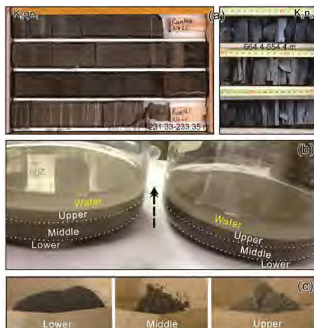
Figure 3. Settling layer-specified character for pulverized oil shales and mudstones from borehole Ngn2, exhibiting photographs of borehole cores (a), grain size separation in the water column for pulverized shales (b), and the powders of layer-specified particles (c).
