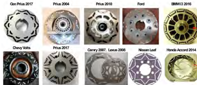
Figure 3. Rotors of electric machines for the recent hybrid electric vehicles (HEVs) and electric vehicles (EVs).
