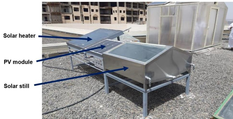
Figure 2. A photo of the designed smart hybrid solar heater–solar still system.
