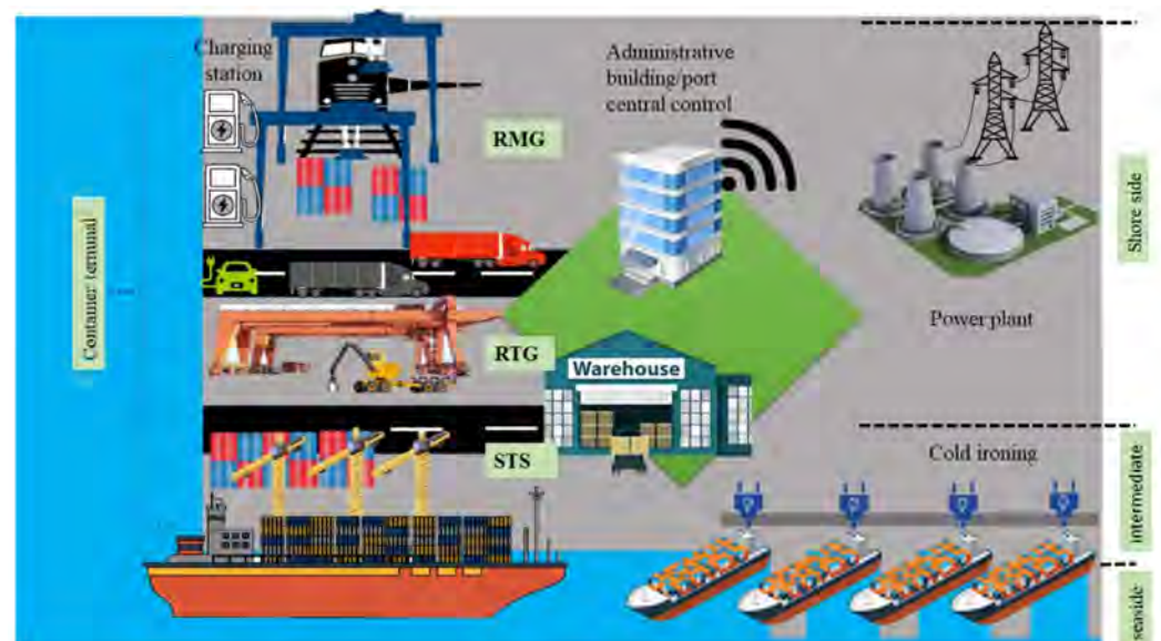
Figure 3. Seaport activities and load components (abbreviations: rail mounted gantry (RMG), rubber tyred gantry (RTG), and ship to shore (STS)).
