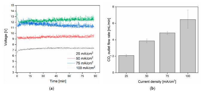
**Figure 2.** (a) Measured voltages for different applied current densities (experimental conditions:  $Q_{inlet} = 20 \text{ mL/min}$ ,  $Q_{pump} = 1 \text{ mL/min}$ ,  $CO_2/N_2$  ratio = 100%/0%). (b) Average  $CO_2$  flow for different applied current densities with the same experimental conditions.
