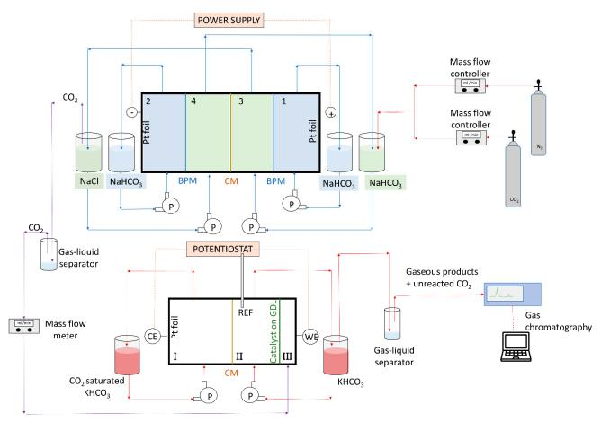
**Scheme 2.** Schematic representation of the coupling between the capture (upper reactor) and the conversion module (lower reactor). P: pump; CM: cationic membrane; BPM: bipolar membrane; CE: counter electrode; WE: working electrode; REF: reference electrode; GDL: gas diffusion layer.
