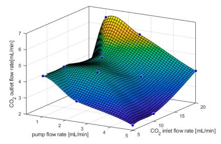
**Figure 6.** Interpolating fit of experimental CO<sub>2</sub> outlet results obtained at  $J = 100 \text{ mA/cm}^2$  for different CO<sub>2</sub> inlet and pump flow rates. The blue points are the experimental data.
