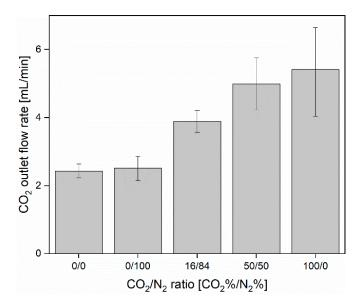
**Figure 5.** Average CO<sub>2</sub> flow for different compositions of inlet gas (experimental conditions:  $Q_{\text{inlet}} = 20 \text{ mL/min}, Q_{\text{pump}} = 5 \text{ mL/min}, J = 100 \text{ mA/cm}^2$ ).
