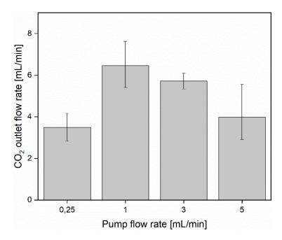
**Figure 3.** Average CO<sub>2</sub> flow for different pump flow rates (experimental conditions:  $Q_{\text{inlet}} = 20 \text{ mL/min}, J = 100 \text{ mA/cm}^2, \text{CO}_2/\text{N}_2 \text{ ratio} = 100\%/0\%$ ).
