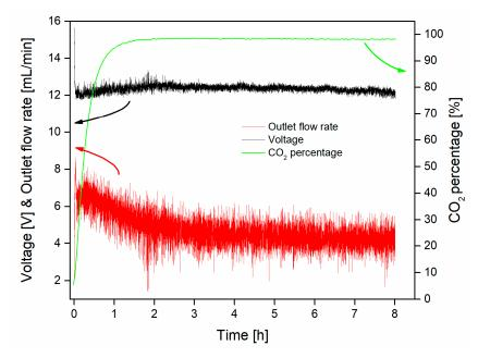
**Figure 7.** Measured voltage (left axis), CO<sub>2</sub> outlet flow rate, and purity of CO<sub>2</sub> in the outlet gas (right axis) during the stability test of eight hours (experimental conditions:  $Q_{inlet} = 20 \text{ mL/min}$ ,  $Q_{pump} = 1 \text{ mL/min}$ ,  $J = 100 \text{ mA/cm}^2$ , CO<sub>2</sub>/N<sub>2</sub> ratio = 100%/0%).
