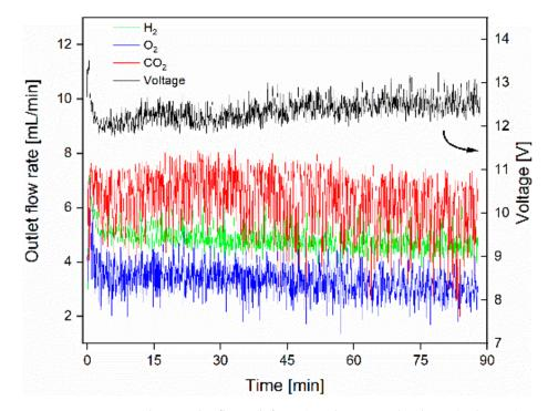
**Figure 1.** CO<sub>2</sub>, O<sub>2</sub> and H<sub>2</sub> outlet flows (left axis) and measured voltage (right axis) in a typical experiment carried out with the capture and release unit (experimental conditions:  $J = 100 \text{ mA/cm}^2$ ,  $Q_{\text{inlet}} = 20 \text{ mL/min}$ ,  $Q_{\text{pump}} = 1 \text{ mL/min}$ , CO<sub>2</sub>/N<sub>2</sub> ratio = 100%/0%).
