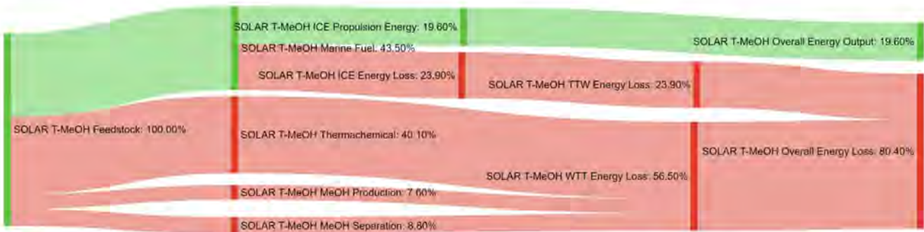
Figure A30. Sankey diagram for methanol produced from solar thermal energy, SOLAR-T-MEOH.
