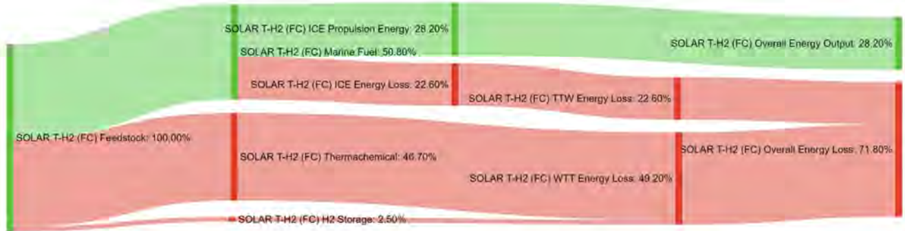
Figure A29. Sankey diagram for hydrogen produced from solar thermal energy, SOLAR-T-H 2 (FC).
