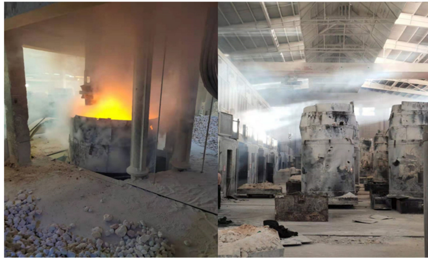
Figure 1. Fused Magnesium Furnace.
