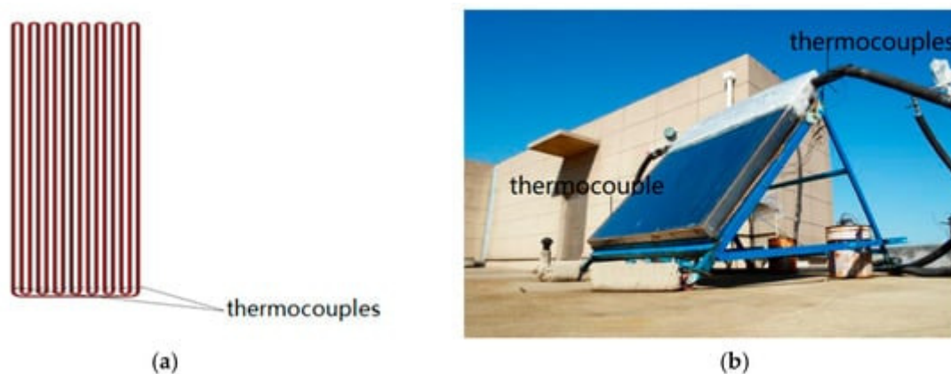
Figure 12. Schematic diagram of main parts and thermocouples' (a) distribution on the absorber and cover (b) (reprinted from Reference [68] under the terms of the Creative Commons Attribution License CC BY 4.0 license, https://creativecommons.org/licenses/by/4.0/ (accessed on 25 October 2021)).
