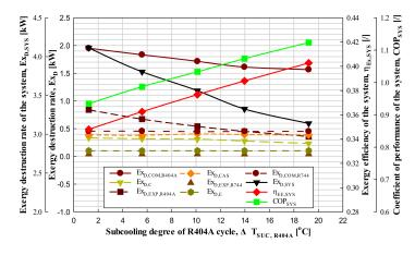
**Figure 4.** Exergy destruction rate, exergy efficiency and COP of the CRS with respect to subcooling degree of R404A cycle.
