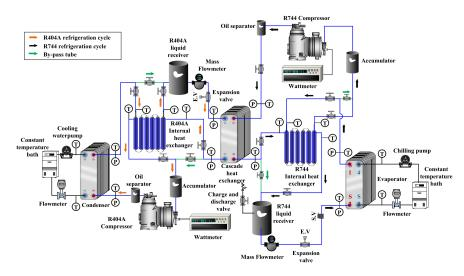
**Figure 2.** Schematic diagram of experimental apparatus for the CRS using R744. [13]. **Table 2.** Experimental conditions of the CRS [13].
