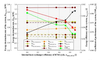
**Figure 11.** Exergy destruction rate, exergy efficiency and COP of the CRS with respect to the IHE efficiency of the R744 cycle.
