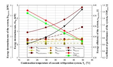
**Figure 7.** Exergy destruction rate, exergy efficiency and COP of the CRS with respect to condensation temperature of the CRS.
