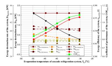
**Figure 8.** Exergy destruction rate, exergy efficiency and COP of the CRS with respect to the evaporation temperature of the CRS.
