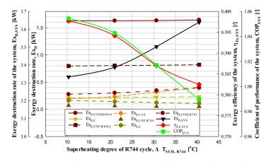
**Figure 6.** Exergy destruction rate, exergy efficiency and COP of the CRS with respect to superheating degree of R744 cycle.
