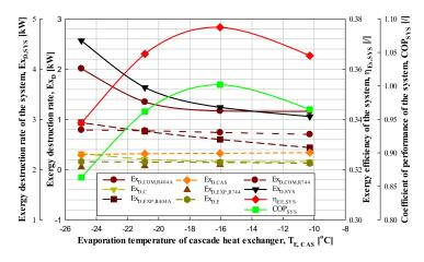
**Figure 9.** Exergy destruction rate, exergy efficiency and COP of the CRS with respect to the evaporation temperature of the cascade heat exchanger.
