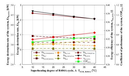
**Figure 12.** Performance analysis results with respect to superheating degree in the R404A cycle of the CRS.
