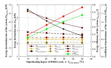
**Figure 5.** Exergy destruction rate, exergy efficiency and COP of the CRS with respect to superheating degree of R404A cycle.
