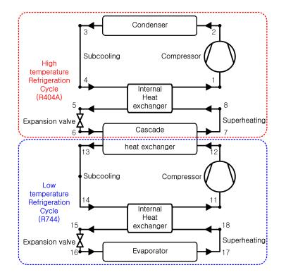
Figure 3. The conceptual diagram of the R744/R404A CRS.
