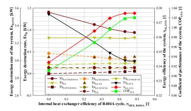
**Figure 10.** Exergy destruction rate, exergy efficiency and COP of the CRS with respect to the IHE efficiency of the R404A cycle.
