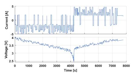
**Figure 11.** First-two dynamic load profiles of the aging cycles applied for model training and validation.
