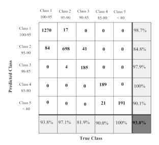
**Figure 17.** Confusion matrix for performance analysis of ANN-based classifier under the step charging current profile validation. The diagonal cells are correctly classified buffers. The last row with gray background is the TPR. The last column with gray background is the precision per class. The bottom right cell with dark background is the total accuracy.
