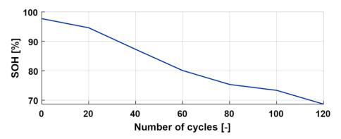
Figure 18. SOH of cylindrical Sanyo NCR 18650 GA lithium-ion cell across the aging cycles.
