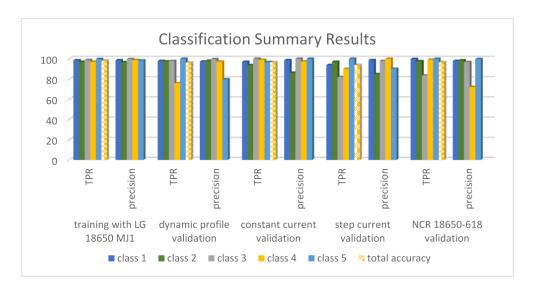
**Figure 20.** Result summary of the training and validation of the classifier indicating the TPR, precision per class, and the total accuracy of the classifier according to the confusion matrices.
