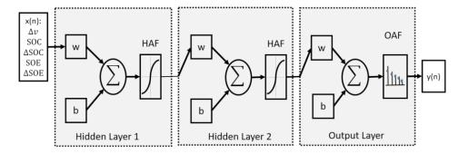
**Figure 9.** Architecture for pattern recognition feed-forward artificial neural network (ANN) for SOH classification. x(n): input; w: weight of layer neurons; b: bias of the layers; HAF: hidden layer activation function; OAF: output layer activation function.
