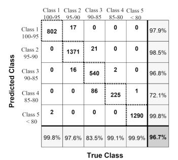
**Figure 19.** Confusion matrix for model validation with NCR 18650 GA lithium-ion cell under dynamic load profile. The diagonal cells are correctly classified buffers. The last row with gray background is the TPR. The last column with gray background is the precision per class. The bottom right cell with dark background is the total accuracy.
