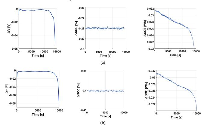
**Figure 8.** Feature extraction across buffer of time length of 40 s. (a) Relative values of voltage, SOC, and SOE in the first cycle. (b) Relative values of voltage, SOC, and SOE in the last cycle.
