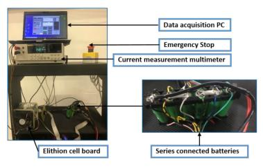
Figure 2. Experimental setup for data acquisition from lithium-ion batteries connected in series.
