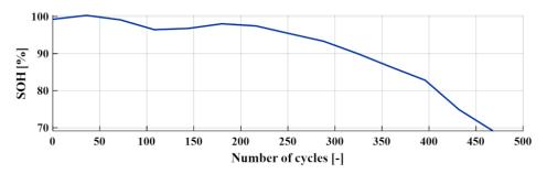
Figure 4. SOH of cylindrical LG MJI 18650 lithium-ion cell across the aging cycles.
