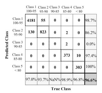
**Figure 15.** Confusion matrix for performance analysis of ANN-based classifier under constant charge current profile validation. The diagonal cells are correctly classified buffers. The last row with gray background is the TPR. The last column with gray background is the precision per class. The bottom right cell with dark background is the total accuracy.
