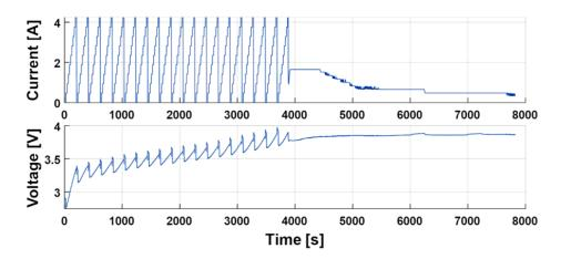
Figure 16. Sample of step charge current profile and the voltage used for model validation.
