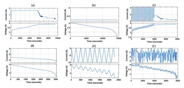
**Figure 3.** Characteristics of the major profiles used for cell aging. (a) constant current (1.75 A) constant voltage charge; (b) constant current (0.7 A) discharge; (c) step current (0 A to 4.23 A) charge; (d) pack constant power discharge (75 W); (e) step current (0 A to -10 A) discharge; (f) dynamic current profile.
