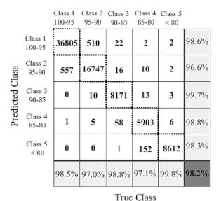
**Figure 12.** Confusion matrix for performance analysis of ANN-based classifier in the dataset trained with LG 18650 MJ1 lithium-ion. The diagonal cells are correctly classified buffers. The last row with gray background is the TPR. The last column with gray background is the precision per class. The bottom right cell with dark background is the total accuracy.
