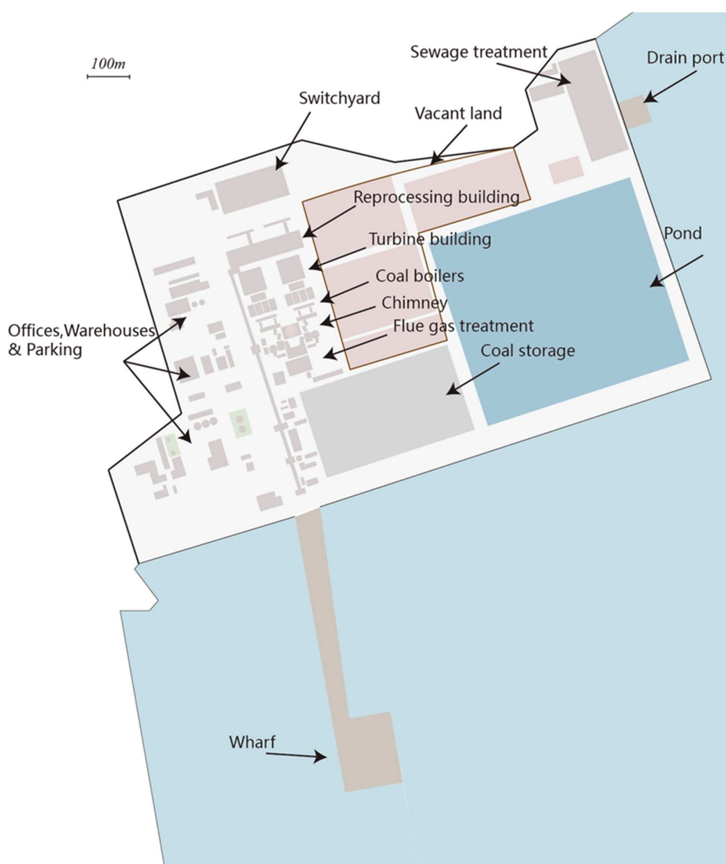
Figure 11. DALIAN Zhuanghe power plant site layout.
