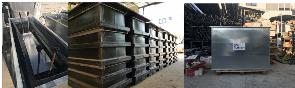
Figure 2. TES tanks (HTES, CTESs or DHW).
