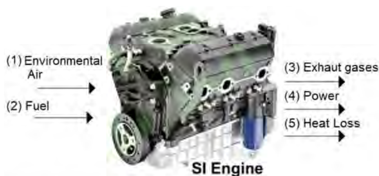
Figure 1. Energy balance in the SI engine.
