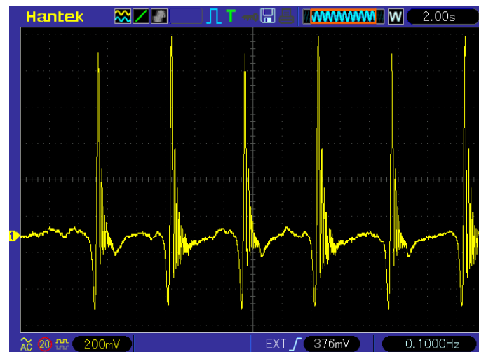
Figure 4. Time dependence of the change in the amplitude of the recorded NMR signal. The modulation frequency of the magnetic field is f_m = 0.1 Hz.
