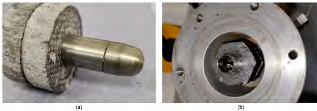
Figure 9. Heat transfer improvements: (a) shows a machined 'bullet' to enable a tighter fit of sample to be pushed over the tube, with the salt composite shown on the tube; (b) shows hexagonal samples inside the shell side LTJ, CALGAVIN insert can be seen within the tube.
