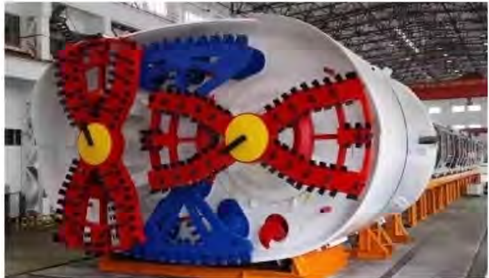
Figure 1. Quasi-rectangular EPB shield machine.
