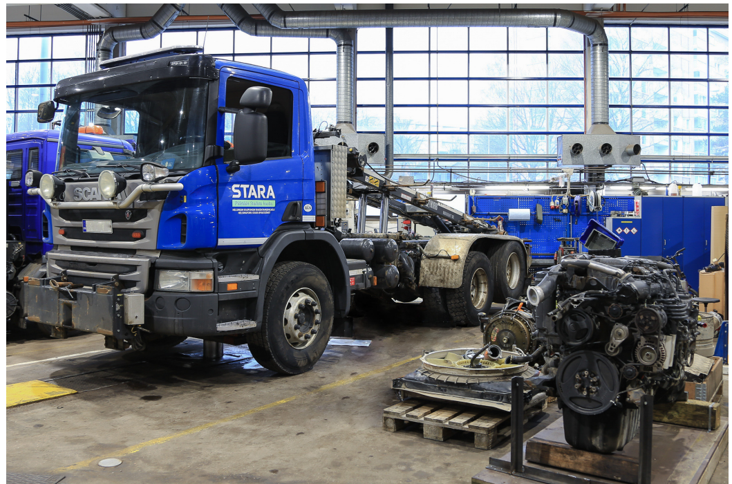
Figure 3. The original diesel truck to be e-retrofitted, together with the removed diesel engine in the lower right corner. Photo credit: Ruska Tapiovaara, Forum Virium Helsinki Ltd., Helsinki, Finland.
