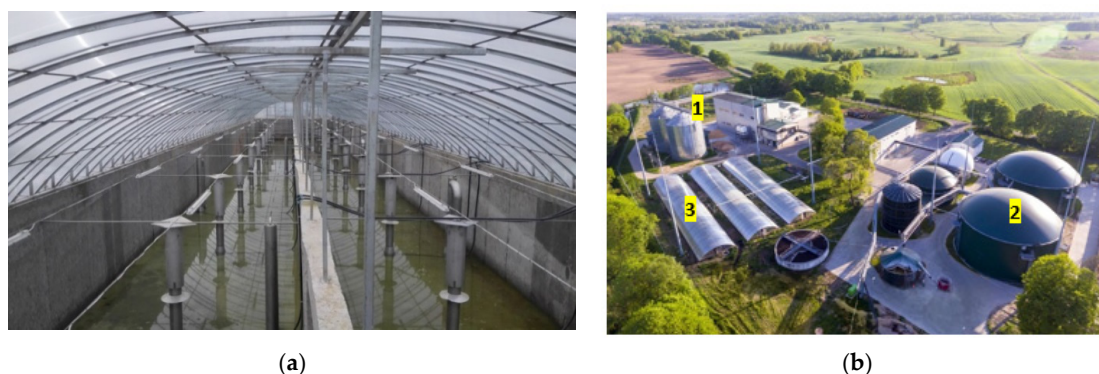
Figure 9. Photobioreactor for growing microalgae based on digestate ((a) overview, (b) placement in the process flow of the biorefinery: 1—distillery, 2—biogas plant, 3—microalgae photobioreactors).
