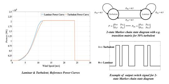
**Figure 5.** Laminar ( $P_{\omega_i} = f_{laminar}(\omega_i)$ ) and turbulent ( $P_{\omega_i} = f_{turbulent}(\omega_i)$ ) power curves and twostate Markov chain state diagram with, e.g., transition matrix for 50% turbulent case.
