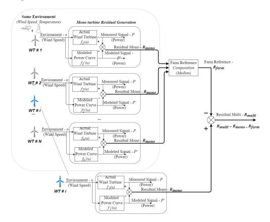
**Figure 2.** Overview of the hybrid multi-turbine approach: generic principle for the synthesis of fault indicator  $R_{multi}$  for wind turbine *i*. The mono-turbine residual  $R_{mono}$  is used for calculating farm reference  $R_{farm}$  and consequently the hybrid mono-multi-turbine residual.
