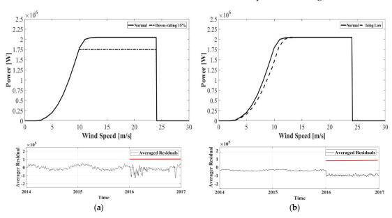
**Figure 7.** Examples of reference fault power curves: (**a**) Down-Rating with power curves for Normal, 15% fault signatures and residual generated for Down-Rating 15% using Method 1 (**b**) Icing with power curves for Normal, icing low fault signatures and residual generated for Icing 5% using Method 1.
