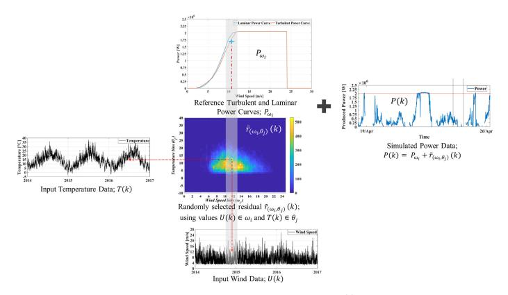
**Figure 4.** Overview of the simulation framework. Power P(k) is simulated by adding data dispersion  $\tilde{r}_{(\omega_i, \theta_j)}(k)$ , randomly selected using input U(k), T(k) pair and reference power curves  $P_{\omega_i}$  (laminar and turbulent).
