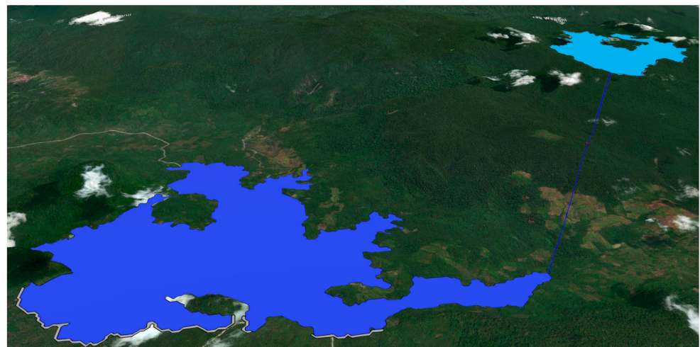
Figure 3. Potential 150 GWh Greenfield off-river pumped hydro energy storage site on Wowonii island near Sulawesi. The upper and lower reservoirs are light and dark blue, respectively. Head: 609 m; separation of reservoirs: 5 km; volume of water: 122 GL (0.8 GL per GWh); combined reservoir area: 1100 Ha (7 Ha per GWh). Latitude/Longitude: 4.21056° S, 123.08990° E. Image from NationalMap [18] and original data from the Australian National University Global Pumped Hydro Atlas [17].
