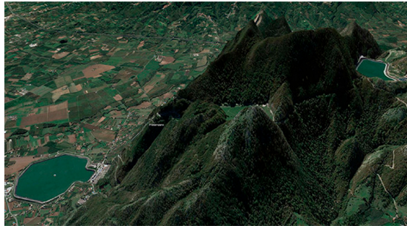
Figure 1. Google Earth synthetic image of a Gigawatt-rated off-river PHEs site at Presenzano in Italy, showing the two reservoirs ( upper right and lower left ) with a head of 500 m (vertical scale exaggerated). Map data ©2021 Google.
