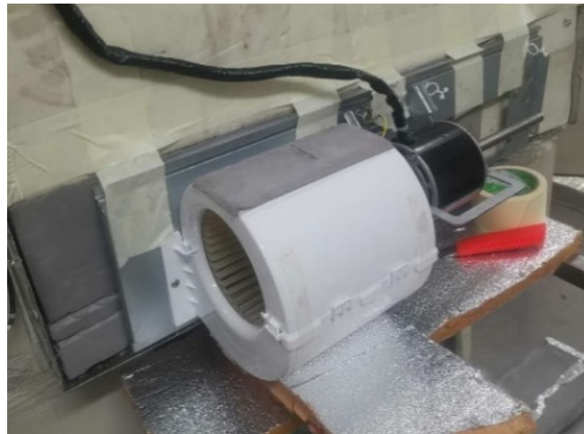
Figure 4. Installation of the tested fan.
