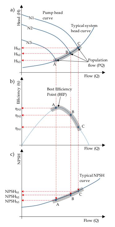
In the building pumping system, the flow demanded by the piping system is modified according to the population's immediate needs (Figure 8; points A, B, and C).
