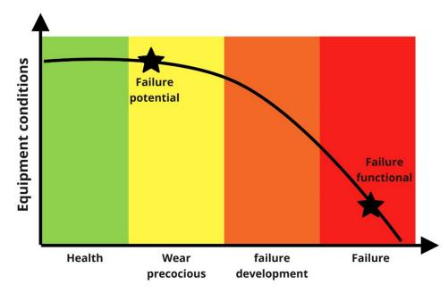
**Figure 3.** PF curve represents the condition of a component until functional failure. Source: Adapted from [52].
