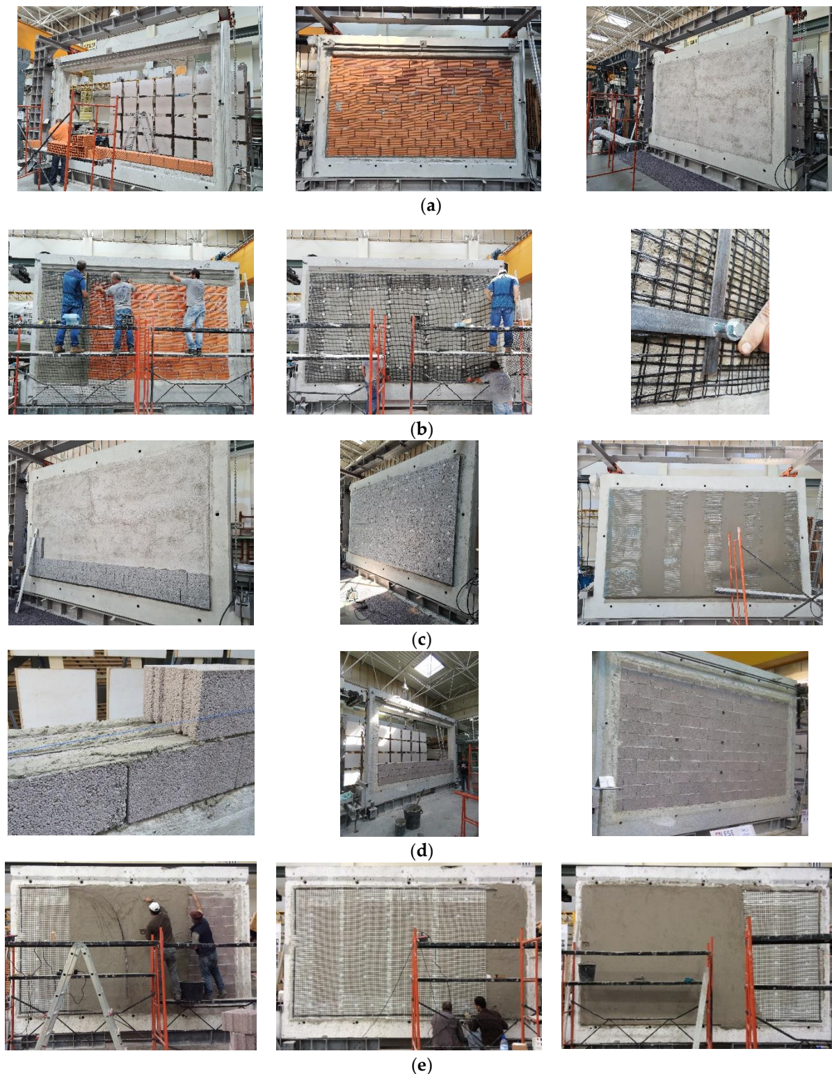
Figure 5. Wall construction procedure: (a) type 1; (b) type 2; (c) type 3; (d) type 4; (e) type 5.
