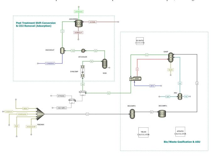
Figure 3. Aspen Plus simulation diagram.
