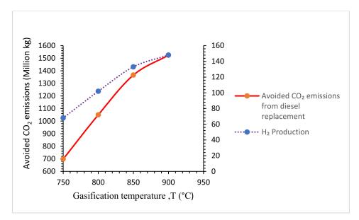
**Figure 9.** Effect of gasification temperature on the level of hydrogen production and the CO<sub>2</sub> emissions avoided.
