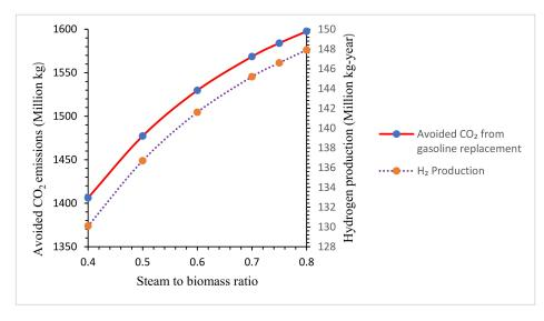
**Figure 11.** Effect of SBTR on CO<sub>2</sub> avoided and hydrogen production.
