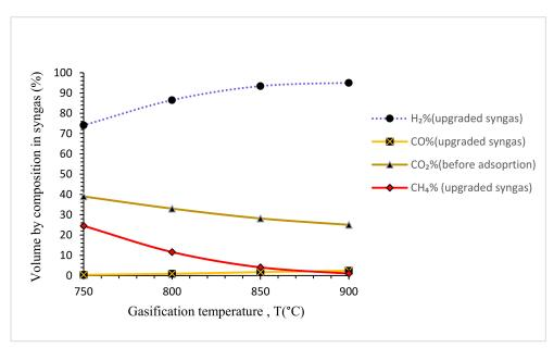
Figure 8. Evolution of syngas composition with gasification temperature.
