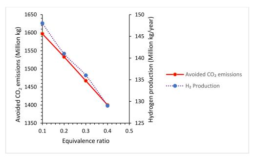
Figure 7. Effect of equivalence ratio on CO<sub>2</sub> avoided and hydrogen production.
