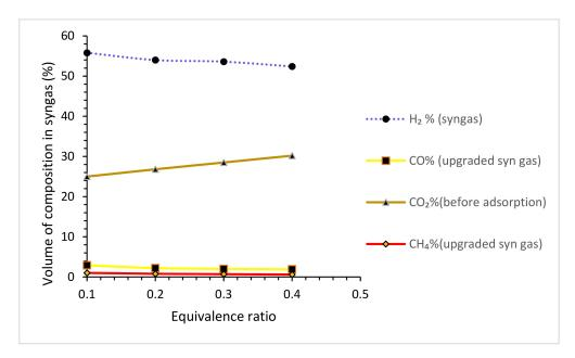
Figure 6. Effect of equivalence ratio on syngas composition.
