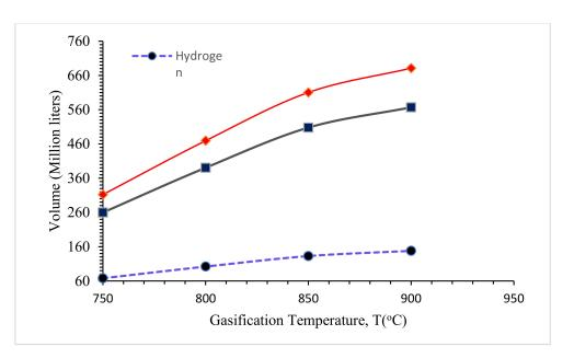
Figure 5. Effect of gasification temperature on hydrogen production and the diesel and gasoline displaced.
