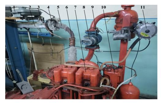
**Figure 3.** Appearance of the hydrogen supply system for the study of the experimental stand performance based on the diesel engine D21A1: 1—tank for liquefied methanol; 2—exhaust manifold of the engine; 3—filter; 4—gas collector; 5—thermal insulation of the exhaust manifold; 6—thermochemical reactor (thermal insulation is partially dismantled); 7—D21A1 diesel engine; 8—gas meter; 9—viewing window in the supply tube of gaseous methanol; 10—high-pressure diesel pump; 11—gas reducer.
