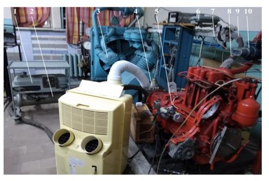
**Figure 2.** Appearance of the experimental stand based on the engine D21A1 for the study of parameters on diesel–hydrogen fuel mixtures: 1—tank for diesel fuel; 2—autonomous heater; 3—load compressor; 4—gearbox; 5—D21A1 diesel engine; 6—tank for methanol; 7—an exhaust manifold of the engine; 8—thermochemical reactor; 9—thermal insulation of the exhaust manifold; 10—gas meter.
