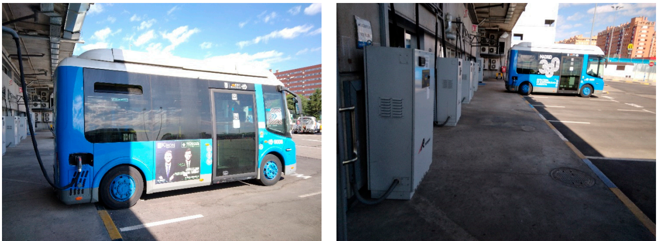
Figure 5. Pictures of wired charging for minibuses in Carabanchel OC (Madrid).
