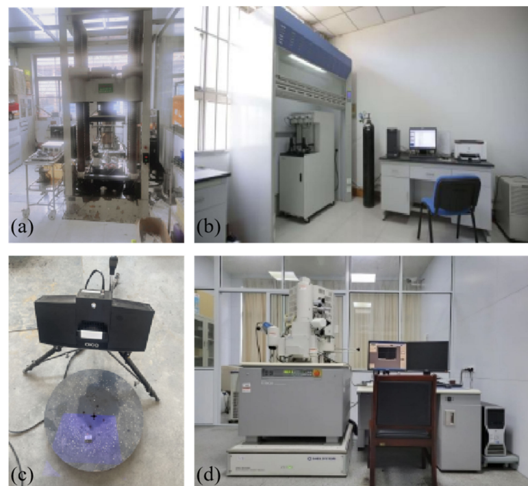
Figure 5. The testing machine: (a) the triaxial testing machine of XTR01-01, (b) the mercury porosimeter of Micromeritics AutoPore V 9620, (c) the 3D scanner of OKIO-3M-400-200-100, and (d) the scanning electron microscope of Hitachi S4800.
