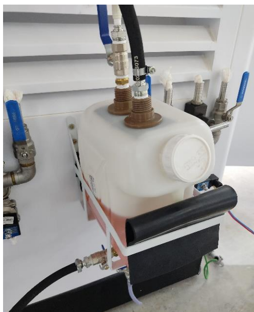
Figure 3. Fixed tank for diesel supply.
