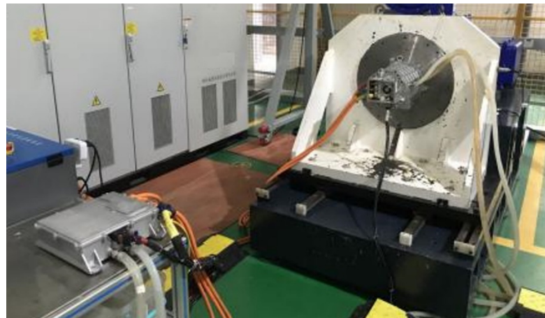
Figure 2. Drivetrain test bench for motor and inverter.
