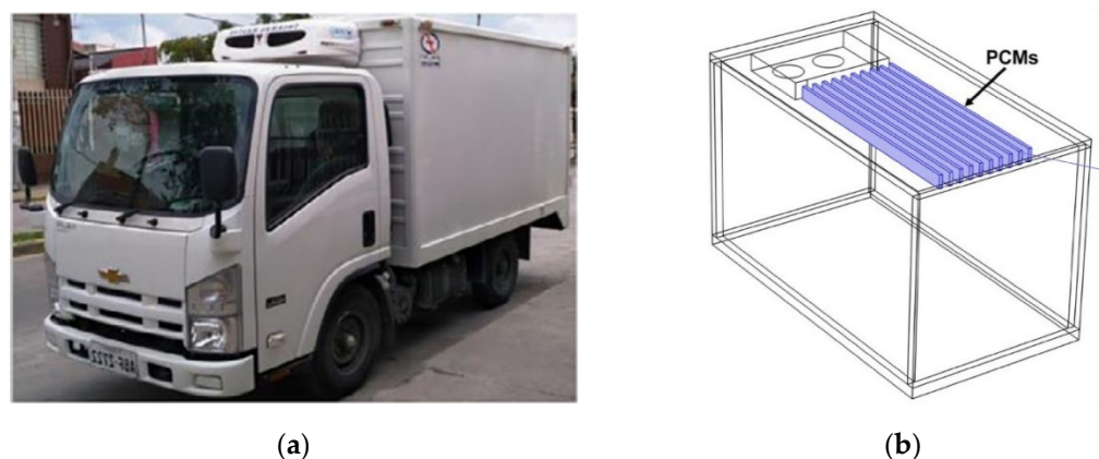
Figure 4. (a) Commercial refrigerated truck; (b) 3D model of the PCM incorporated truck [75].
