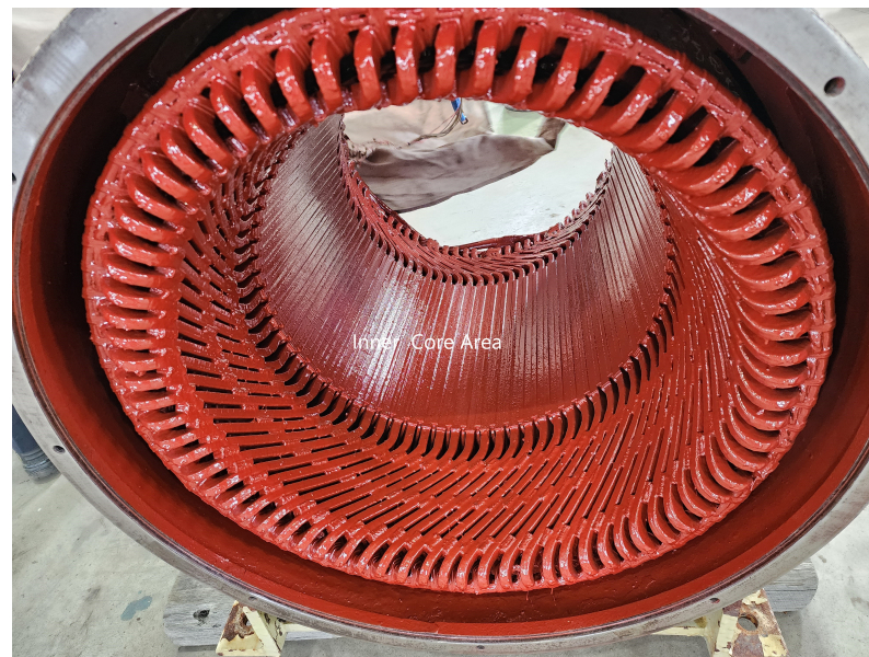
Figure 5. Motor Stator Inner Core Area with Winding.
