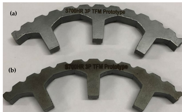
Figure 20. Comparison between TFM segments, (a) machine brushed version for burrs, (b) manual de-burring.
