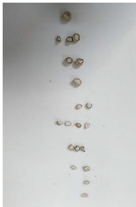
Figure 2. Appearance of large and small balls that formed in a fluidized bed of quartz sand when pellets from sunflower husks were burned in it.
