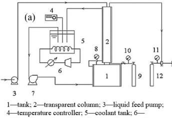
refrigeration system; 7—coolant recycle pump; 8, 10,11—pressure gauge; 9—gas feed cylinder; 12—gas recovery cylinder.
