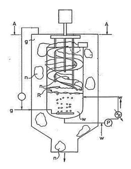
**Figure 14.** MES gas hydrate formation equipment [152]. Where, g: Gas supplied, w: water, n: hydrate sulray, R: Liquid-gas interface.
