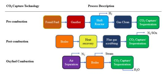
Figure 2. Carbon capture processes.
