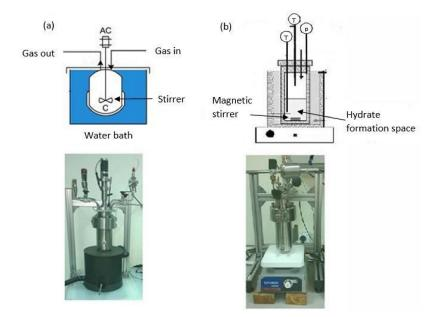
**Figure 4.** Lab-scale stirrer-tank reactors. (a) Impeller and external motor. (b) Magnet bar and magnet stirrer. Pictures are from Phase Separation Laboratory, RCCO<sub>2</sub>C, Universiti Teknologi PETRONAS.
