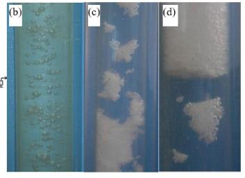
**Figure 6.** (**a**) Schematic drawing of the experimental setup employed by Luo et al. [122]. (**b**) Bubbles without hydrate. (**c**) Bubbles with hydrate cover. (**d**) Hydrate blockage in the reactor.
