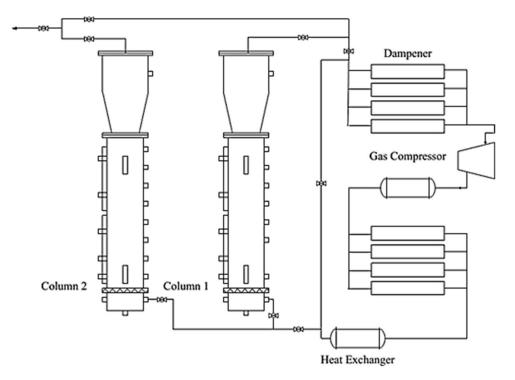
Figure 7. Slurry bubble column setup used by Hashemi et al. [123].
