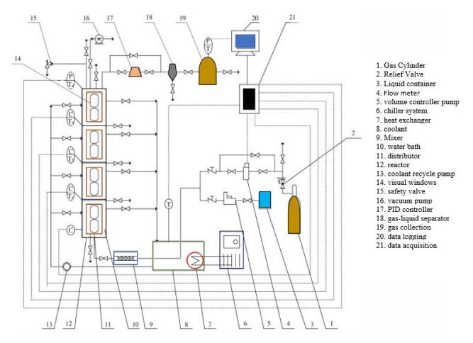
Figure 8. Schematic of experimental apparatuses used by Xu et al. [139].
