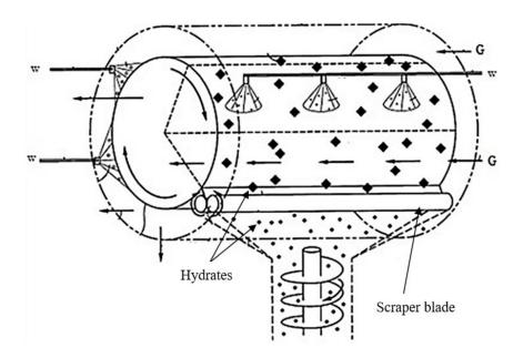
Figure 11. Hydrate production reactor by Heinemann et al. [148]. Where, G: gas, and w: water.
