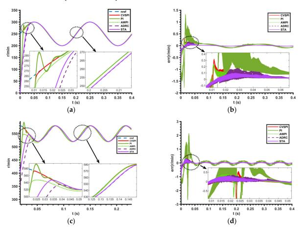
Figure 8. (a) Estimated and actual rotational speeds for the first sine case. (b) The speed error for the first sine case. (c) Estimated and actual rotational speeds for the second sine case. (d) The speed error for the second sine case.
