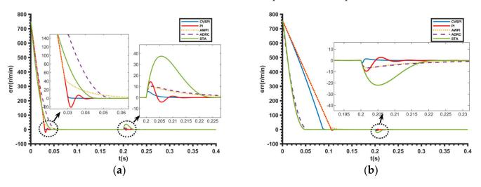
Figure 9. (a) Speed error during sudden load application. (b) Speed error during sudden load discharge.
