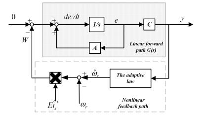
Figure 6. Block diagram of the error system architecture.
