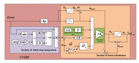
Figure 3. Block diagram of the novel CVSPI controller architecture.
