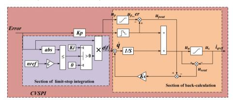
Figure 1. Block diagram of the CVSPI controller architecture.
