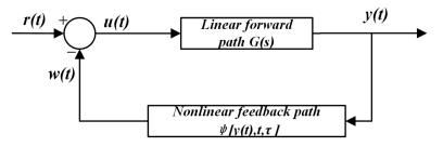
Figure 5. Block diagram of the structure of a non-linear feedback system.
