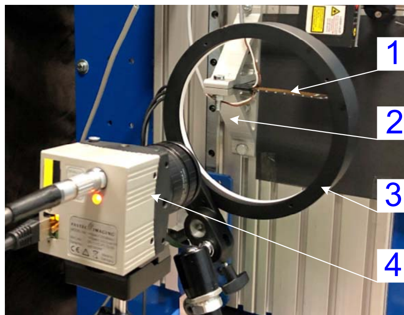
Figure 5. View of main parts of laboratory stand: 1—piezoelectric actuator, 2—clamping assembly, 3—diode illuminator, 4—camera.
