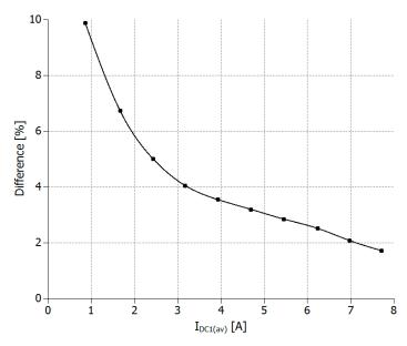
Figure 13. Difference between the measured and estimated average value of the input current  $i_{DC1}$ .
