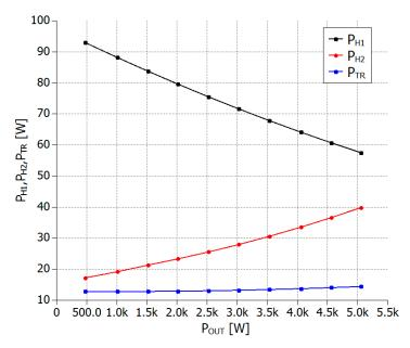
**Figure 15.** The estimated power loss distribution of the tested DAB converter.
