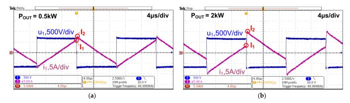
**Figure 16.** Experimental waveforms of the current  $i_1$  and voltage  $u_1$  measured for: (a)  $P_{OUT} = 0.5$  kW; (b)  $P_{OUT} = 2$  kW.
