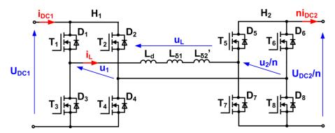
Figure 2. Equivalent circuit of the single-phase DAB converter.
