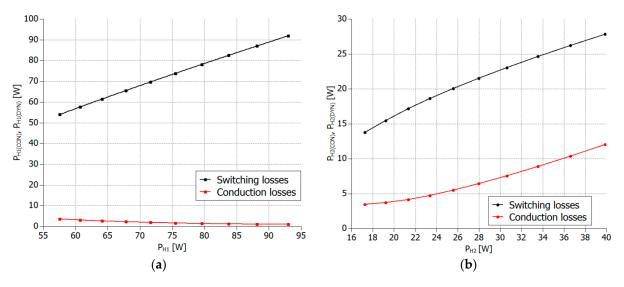
**Figure 17.** Estimated power loss distribution in the considered DAB converter bridges: (a) bridge  $H_1$ ; (b) bridge  $H_2$ .
