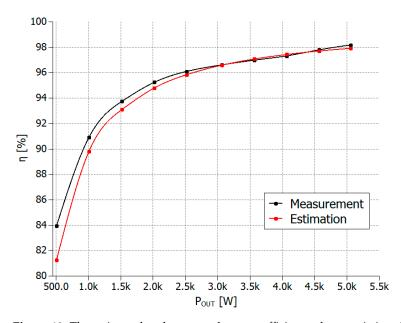
**Figure 19.** The estimated and measured energy efficiency characteristics of the tested DAB converter for the case when energy is transferred from bridge  $H_2$  to  $H_1$ .
