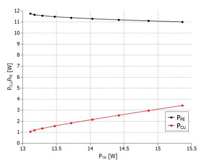
**Figure 18.** The estimated transformer power loss distribution in the DAB converter.
