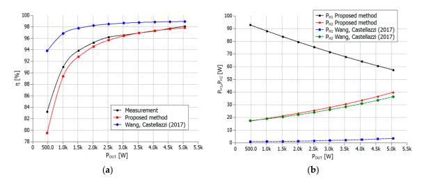
**Figure 20.** Comparison of the results obtained using the proposed method and approach presented by Wang and Castellazzi in [19]: (a) estimated and measured energy efficiency characteristics of the tested DAB converter; (b) power loss characteristics of bridges  $H_1$  and  $H_2$ .
