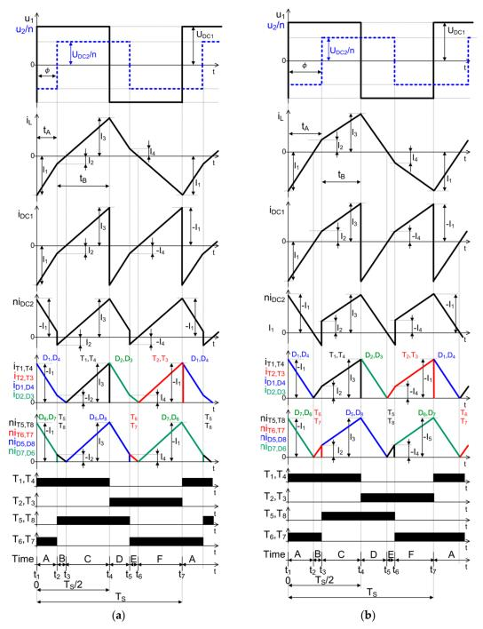
**Figure 3.** Simplified voltage and current waveforms of DAB converter for  $U_{DC1} > U_{DC2}/n$ : (a) with  $I_2 < 0$ ; (b) with  $I_2 > 0$ .
