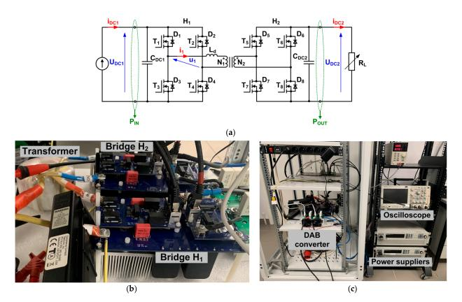
**Figure 12.** Laboratory setup for the experimental tests: (a) Scheme; (b) tested DAB converter; (c) laboratory stand.
