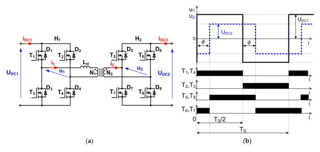
Figure 1. (a) Dual active bridge DC/DC converter topology; (b) single phase shift modulation scheme.
