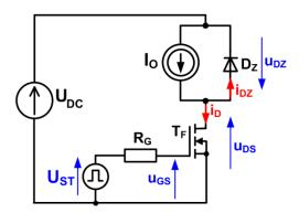
**Figure 6.** Basic switching cell.
