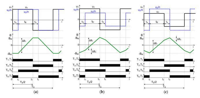
**Figure 11.** Simplified waveforms of voltages  $u_1$ ,  $u_2/n$  and magnetic induction B for (a)  $U_{DC1} = U_{DC2}/n$ ; (b)  $U_{DC1} > U_{DC2}/n$ ; (c)  $U_{DC1} < U_{DC2}/n$ .
