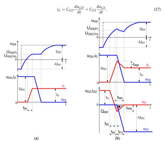
**Figure 7.** Voltage and current waveforms in a basic switching cell during transistor turn-on process: (a) without the diode  $D_Z$  reverse recovery; (b) with the diode  $D_Z$  reverse recovery.
