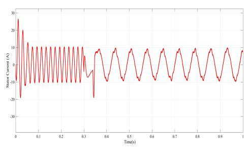
Figure 11. Stator current response to varying load torque.
