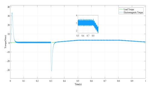
Figure 9. Electromagnetic torque response to step change in speed reference and load torque.
