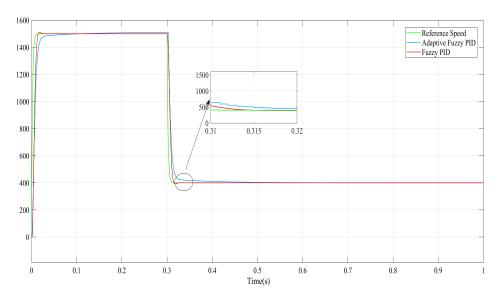
Figure 12. Measured speed response to step change with speed reference when speed decreased.
