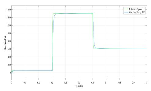
Figure 6. Adaptive fuzzy PID speed controller.
