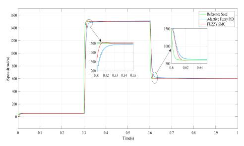
Figure 16. Measured speed to step change with controllers.
