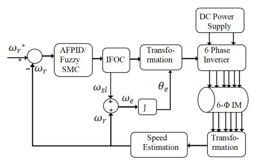
Figure 2. A block diagram of sensorless speed control for six-phase induction motor.
