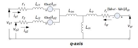
**Figure 1.** Dynamic equivalent circuit of the six-phase induction motor in an arbitrary reference frame [19]. (a) q-axis equivalent circuit of the six-phase induction motor. (b) d-axis equivalent circuit of the six-phase induction motor.
