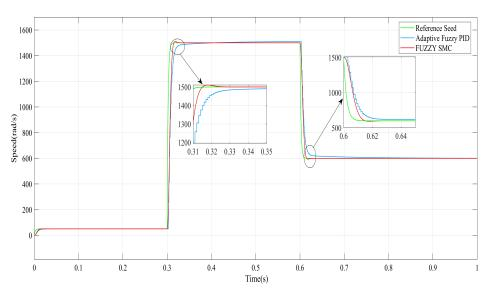
Figure 8. Measured speed response to step change with reference speed when speed increased.
