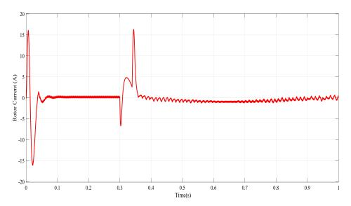
Figure 10. Rotor current response to varying load torque.
