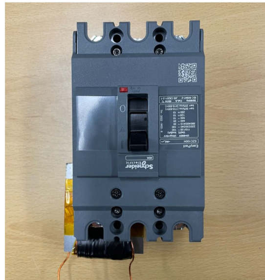
Figure 9. Structure for applying external magnetic field and the circuit breaker.
