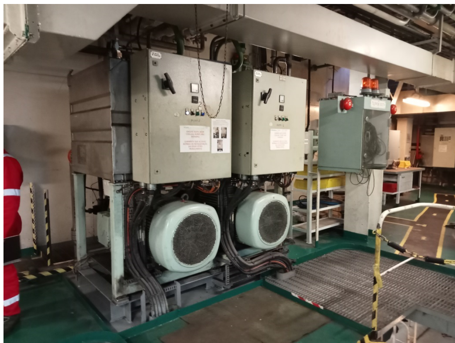
Figure 1. Typical view on the hydraulic twin-two-pump power pack unit on board of the sea ship. Source: shipyard's own documentation.
