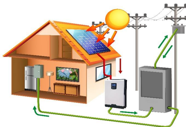
Figure 1. Structure of a typical nanogrid system.
