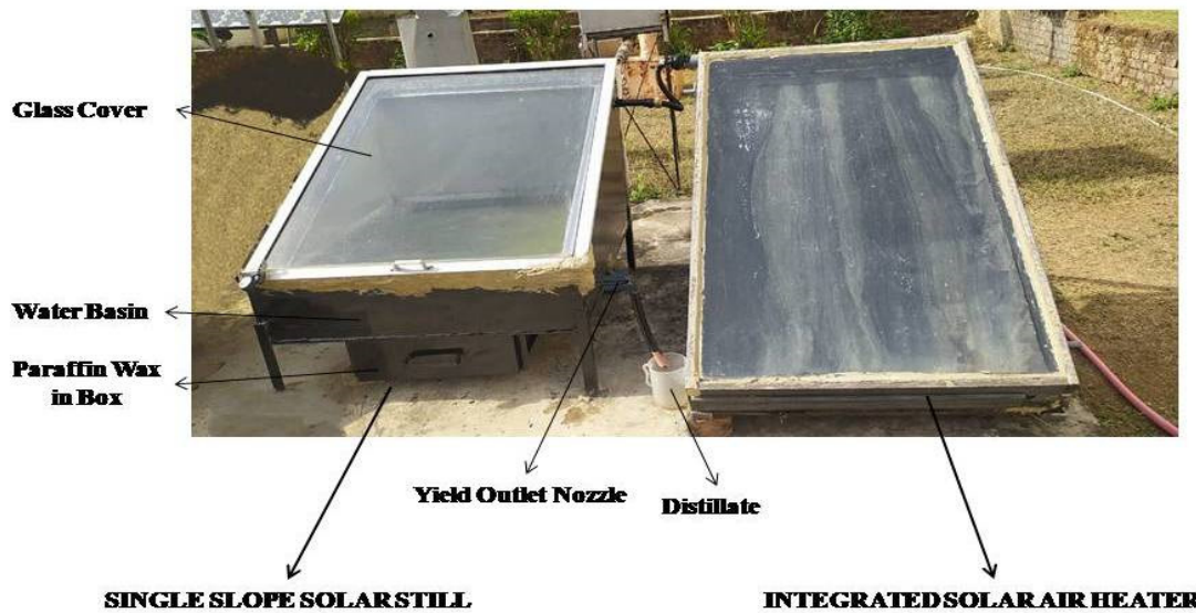
Figure 2. Experimental View of Latent Heat Storage Based Single-Slope Solar Still Assisted with Solar Air Heater.
