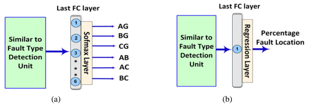
Figure 6. Schematic diagram of (a) the fault classification unit and (b) the fault location estimation unit.
