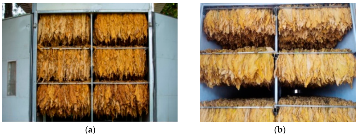
Figure 9. Appearance of tobacco leaves after curing with (a) TCCB and (b) HPCB modes.
