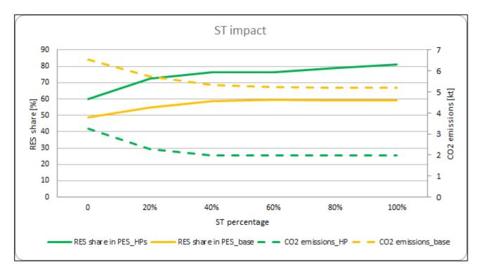
**Figure 12.** Analysis of the impact of solar thermal collectors on the system emissions (right axis) and RES share in PES (left axis).
