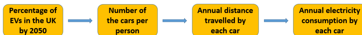
Figure 3. The schematic of the method used for calculation of EVs energy consumption.
