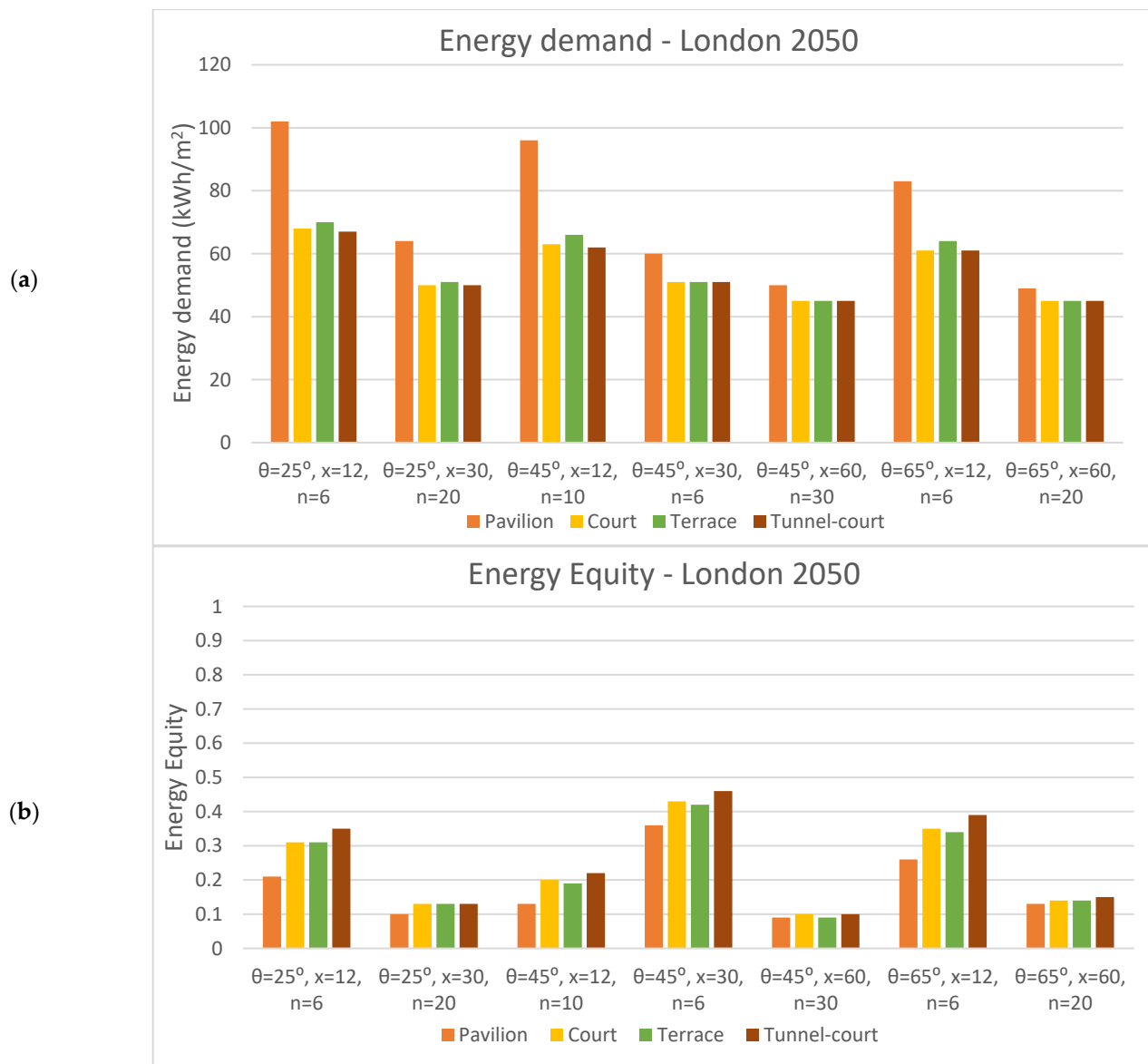
Figure 9. Comparison of the predicted building energy performance of the studied built forms with the same cut-off angles, plan depths and number of storeys in London 2050: (a) energy demand and (b) Energy Equity.
