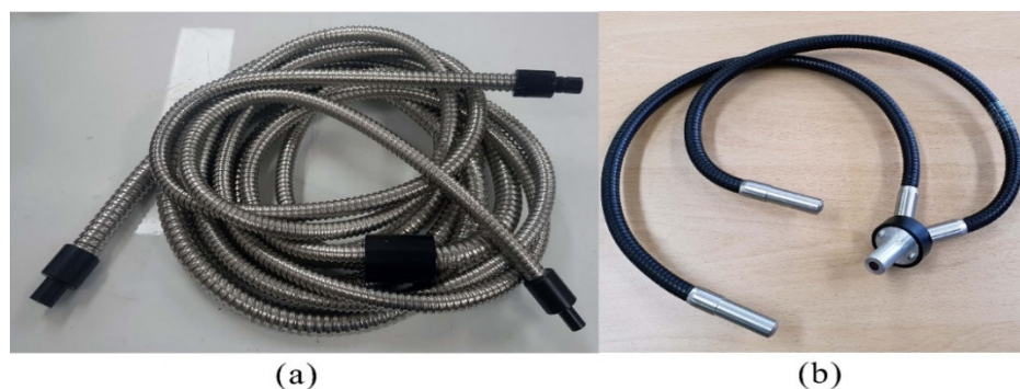
Figure 3. Optical fiber light guides used in the experiment, (a) a glass type light guide; (b) a polymer type light guide.
