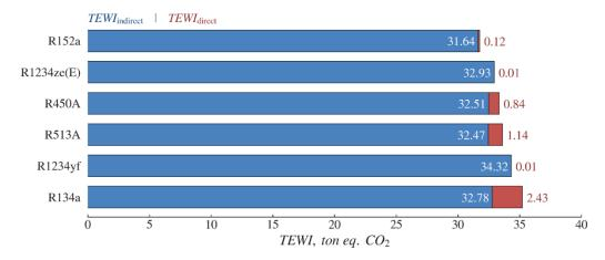
Figure 18. Total equivalent warming impact for different refrigerants.
