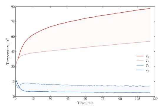
Figure 5. Temperatures measured for refrigerant R134a vs time.
