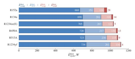
Figure 14. Exergy destructions of the components and cycle for different refrigerants.
