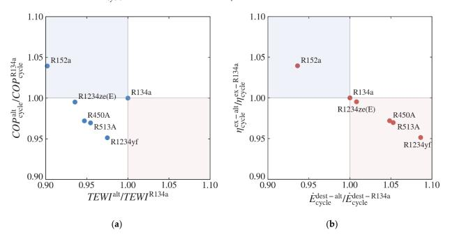
**Figure 19.** Normalized cycle parameter dependences for different refrigerants: (**a**) Coefficient of performance vs. total equivalent warming impact; (**b**) Cycle efficiency vs. exergy destruction.
