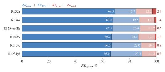
Figure 15. Relative exergy destructions of the components and cycle for different refrigerants.
