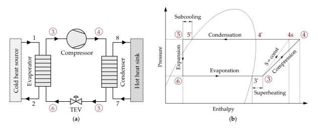
**Figure 3.** Schematic representation of the thermodynamic model: (**a**) Water-to-water heat pump; (**b**) Pressure-enthalpy diagram.
