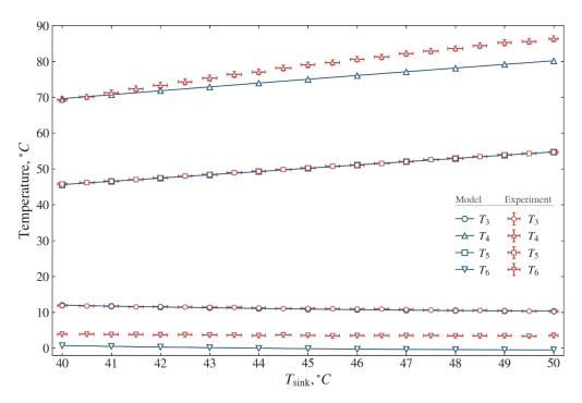
Figure 9. Comparisons of predicted and measured temperatures with the temperature of the heat sink.
